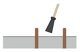
**1.** Clean the surface. All loose particles can negatively affect the bonding to the surface.
