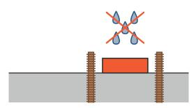
**6.** Protect **SUPROBAND ACR** the gainst water (e.g. rain) until the concrete is placed.
