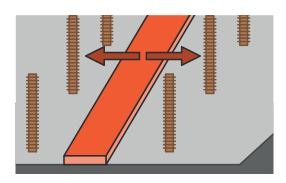
**4.** Press the **SUPROBAND ACR** into the applied adhesive. It is important to get a full bonding to the surface.
